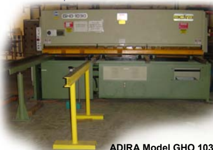
ADIRA Model GHO 1030 Squaring Shear Capacity 10' x 3/8"
